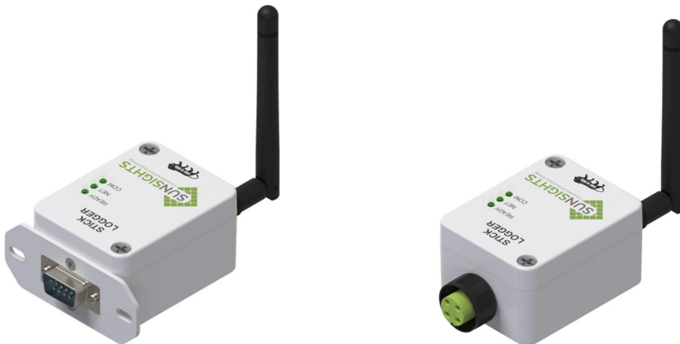
The SunSights Wi-Fi Dongle is designed to establish a seamless connection with a variety of String Inverters equipped with circular connectors/DB9, as illustrated in the accompanying images. To ensure a successful installation, please follow the steps outlined below.
