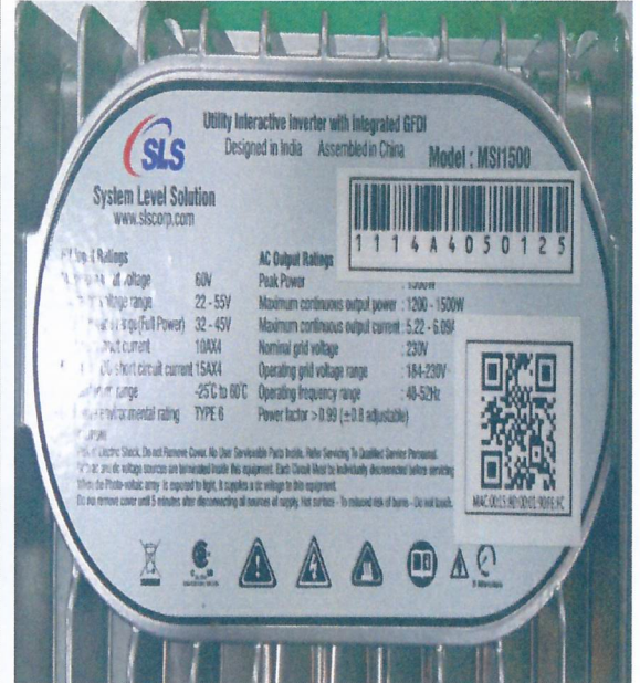
2.Nameplate of inverter
