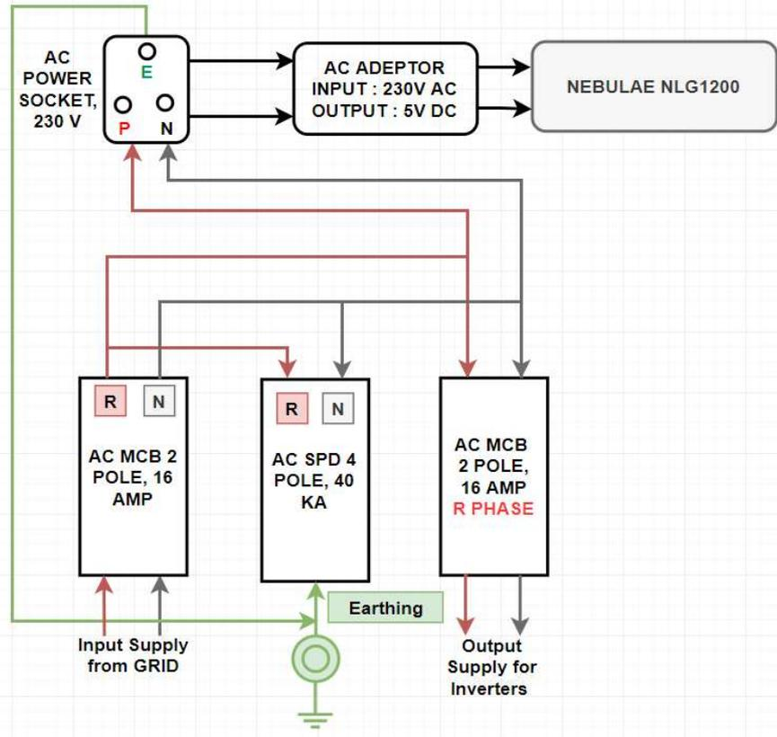
Diagram 4-1: Electrical connection diagram for 1 Phase ACDB
