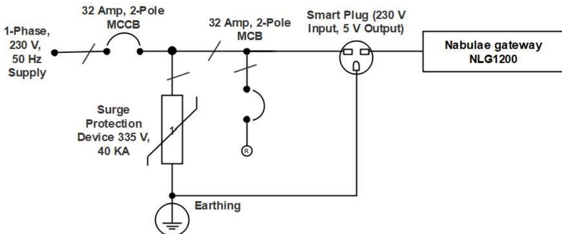
Diagram 5-1: Single Line Diagram for 1 Phase ACDB
